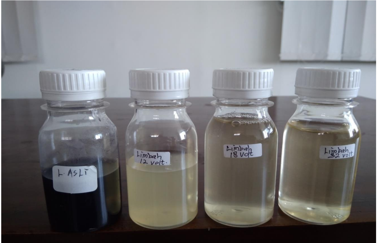
Figure 3. Results of batik waste treatment (a). The original batik waste before being processed, (b) 12 volts, (c) 18 volts, (d) 32 volts.
